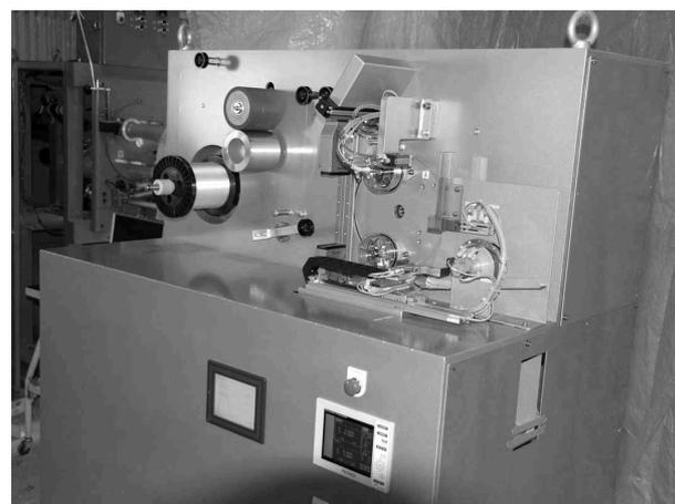
Fig. 9. SPM05-02: a perfect layer winder system with an FPGA control board.
